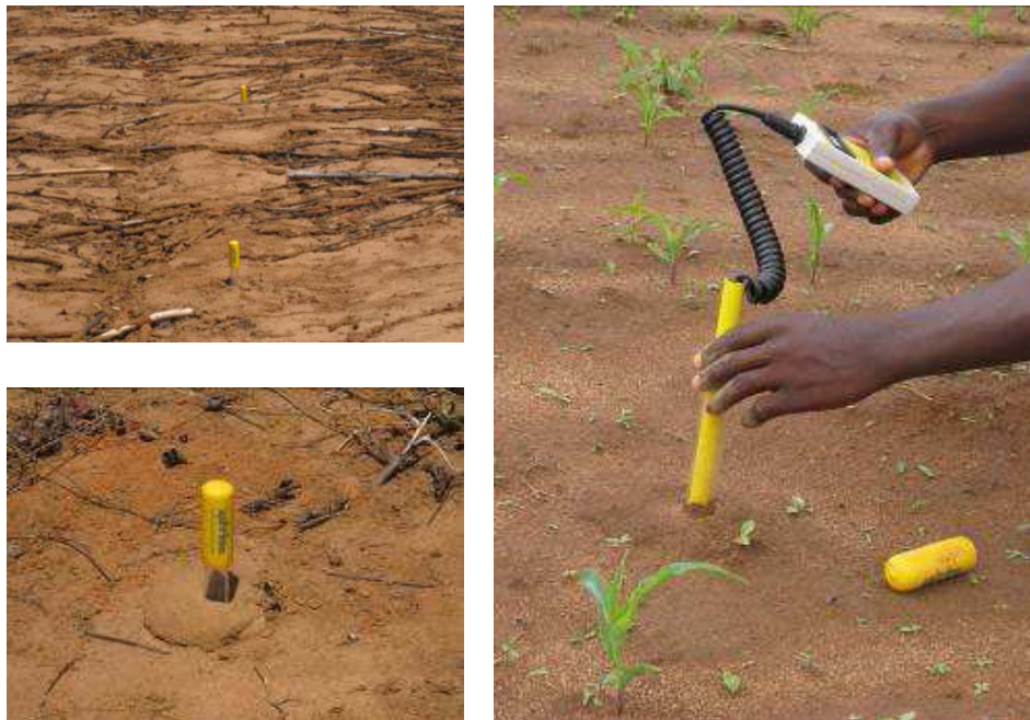
Figure 3.21: Photos showing the installed access tubes in the trial plots (left, up and down) and readings details with AquaPro probes (right).
