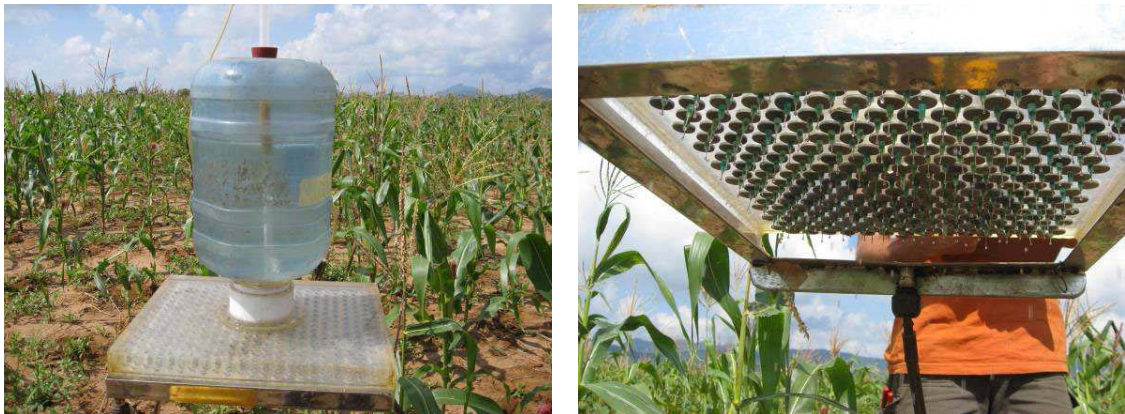
Figure 3.23: Mini-rainfall simulator used in the study, evidencing the Mariotte flask (left), and syringes arrangement (right).
